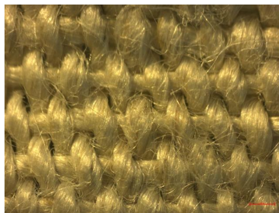
Figure 2 Linen cloth woven in tabby weave. 56g of tension per thread. Photo credit Jennifer Beamer.
