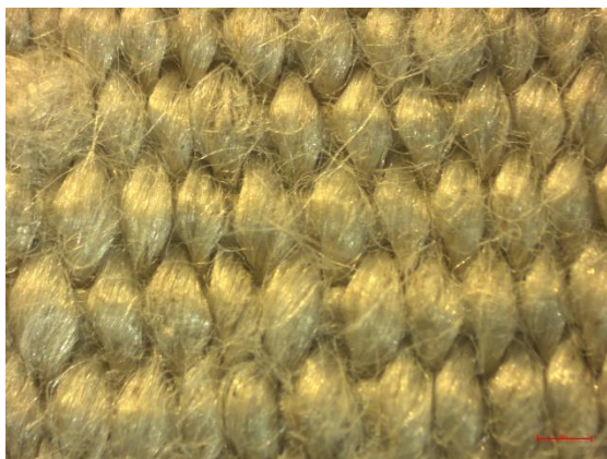
Figure 1 Linen cloth woven in tabby weave. 28g of tension per thread. Photo credit Jennifer Beamer.
